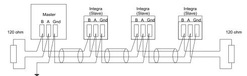
There must be no more than two wires connected to each terminal, this ensures that a "Daisy Chain or "straight line" configuration is used. A "Star" or a network with "Stubs (Tees)" is not recommended as reflections within the cable may result in data corruption.
